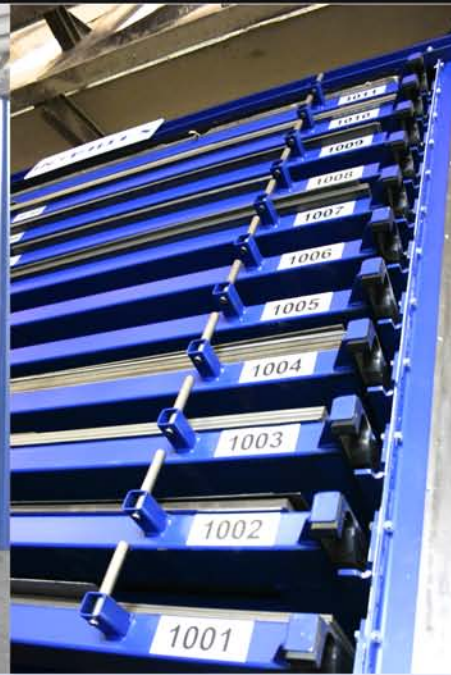
A tight grid allows the flexible allocation of storage bins for different loading heights.
