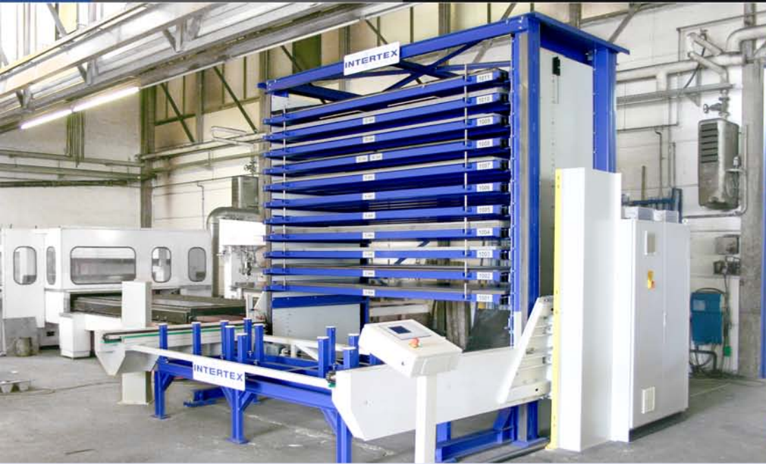
This INTERTEX sheet metal storage system TM EE1.1 can hold 11 storage pallets. These include the placement of the sheet stock for the laser next to it. New sheet metal packages can be stored immediately upon delivery.
